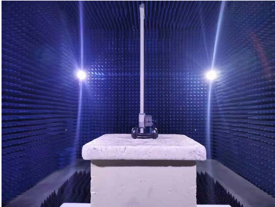
Photo of Radiated Emission Measurement Above 1GHz
