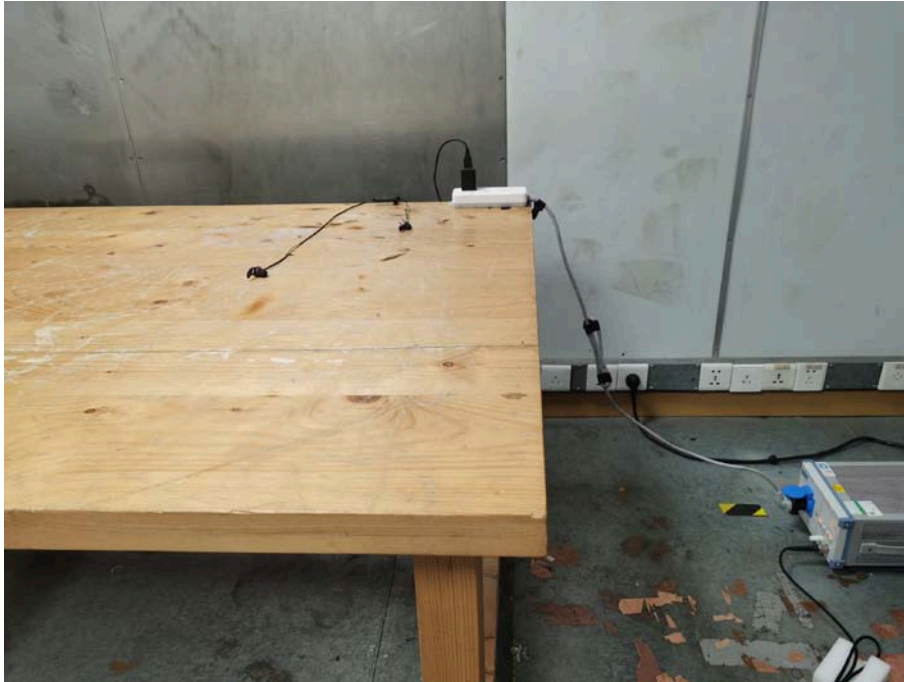
Photo of Power Line Conducted Emission Measurement
