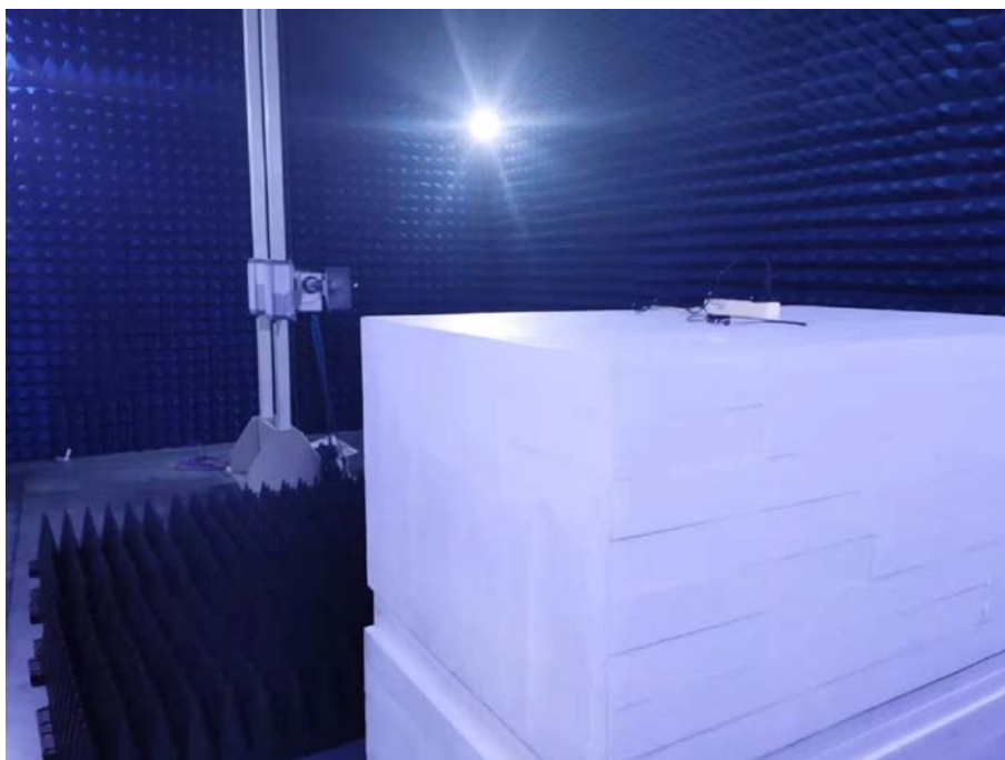
Photo of Radiated Emission Measurement Above 1GHz
