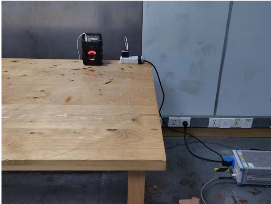
Photo of Power Line Conducted Emission Measurement
