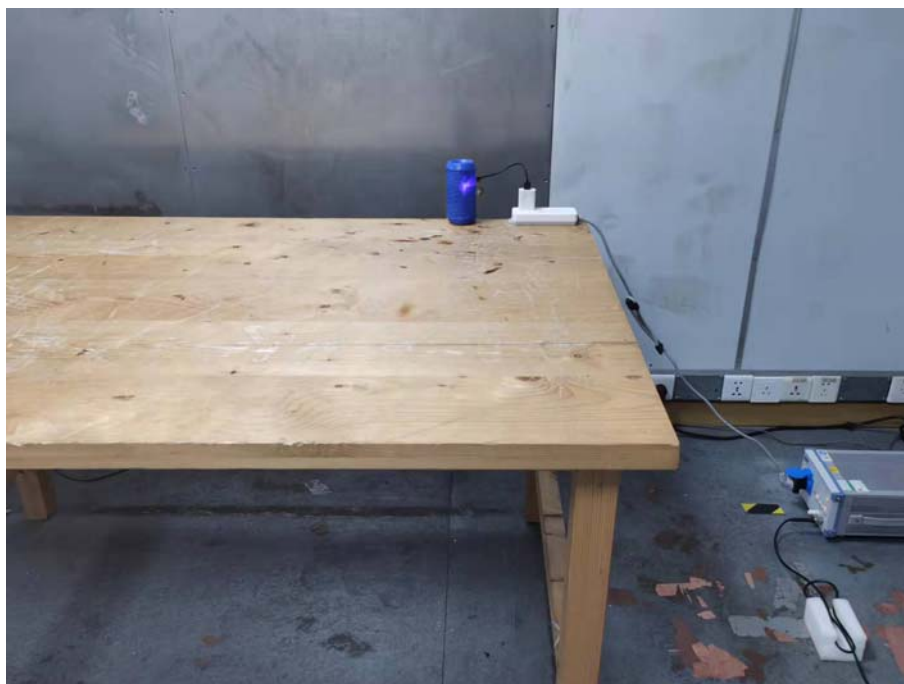
Photo of Power Line Conducted Emission Measurement
