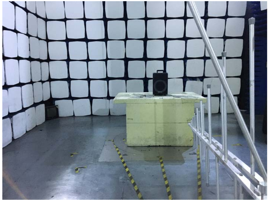
Radiation Emission Test Setup (30MHz to 1GHz)
