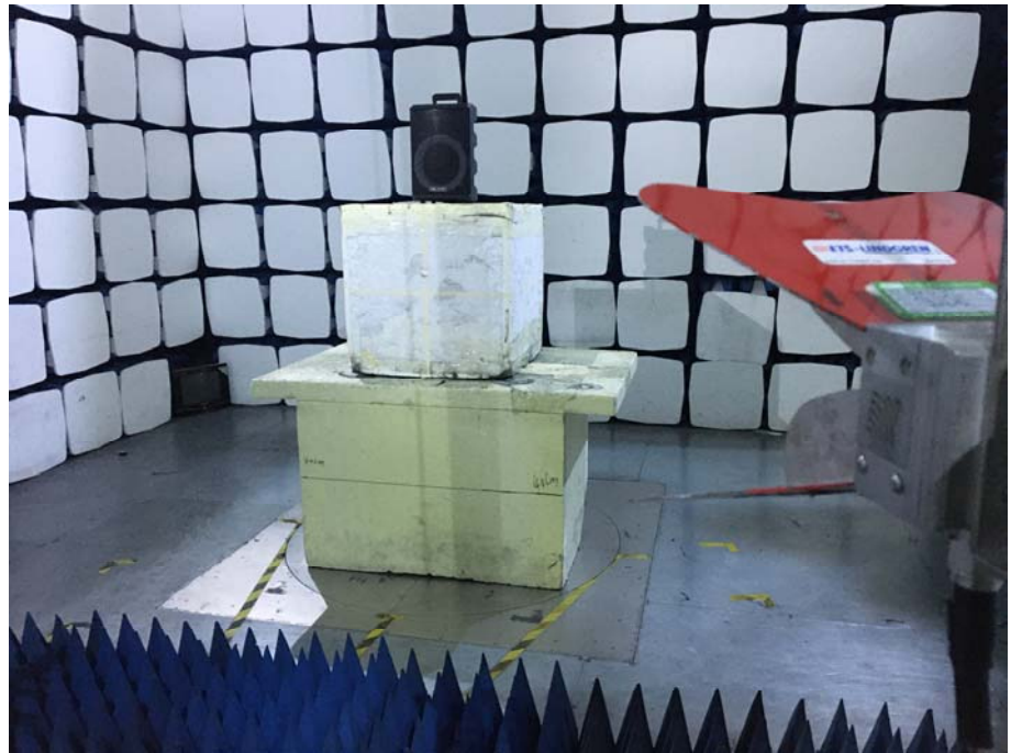
Radiation Emission Test Setup (1GHz to 18GHz)
