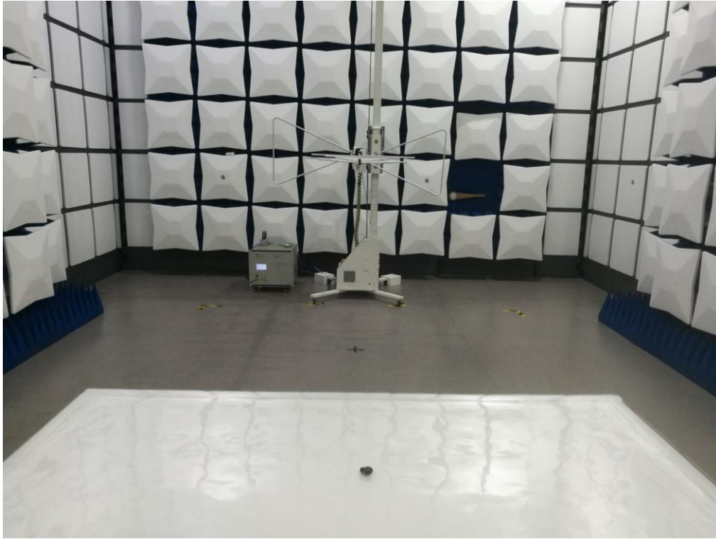
FCC RADIATED EMISSION TEST SETUP
