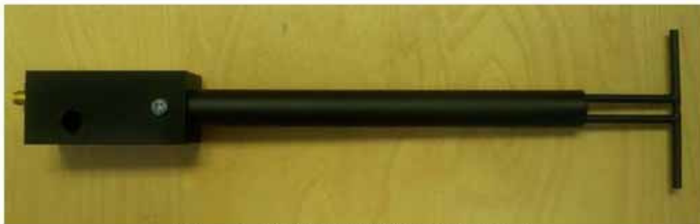
Figure 1 – MVG COMOSAR Validation Dipole
