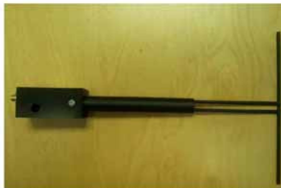
Figure 1 – MVG COMOSAR Validation Dipole
