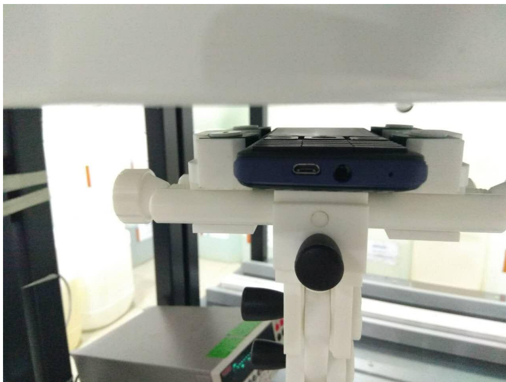
Body Front side(separation distance is 10mm)
