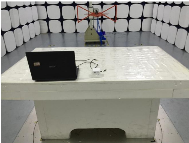
Radiated Spurious Emissions Test Setup Below 1GHz
