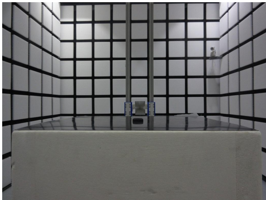
Radiated Spurious emission test above 1GHz
