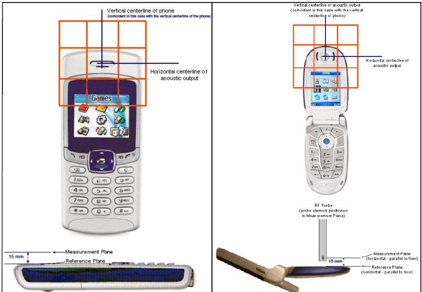
Fig-3.4 EUT Reference and Plane
