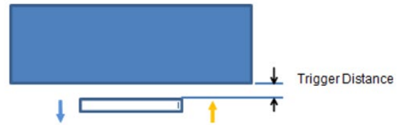
Proximity sensor triggering distances assessment Front/Back side
