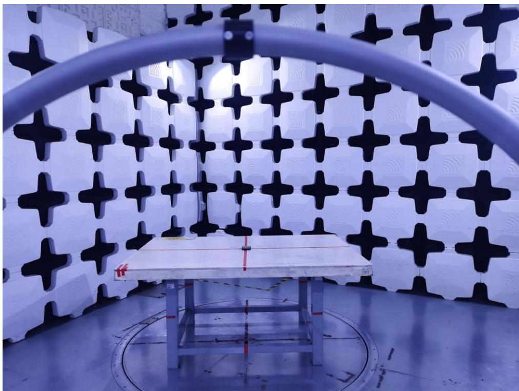
**Radiated Emissions Test Photos****30 MHz to 1 GHz**
