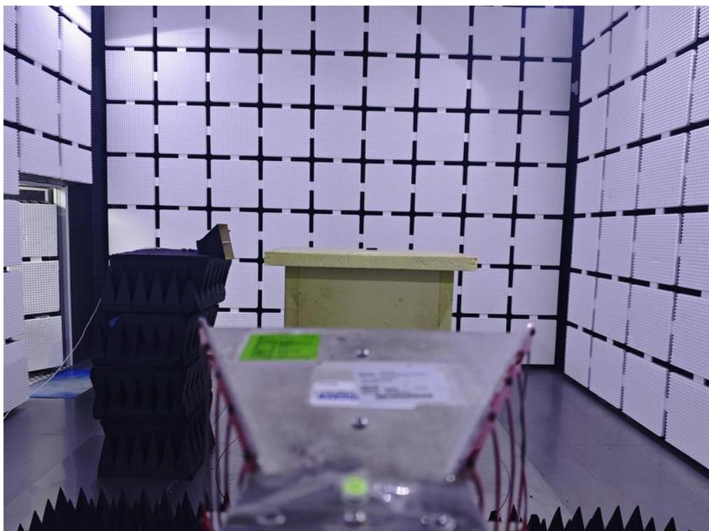
**Radiated Emissions Test Photos****Above 18 GHz**
