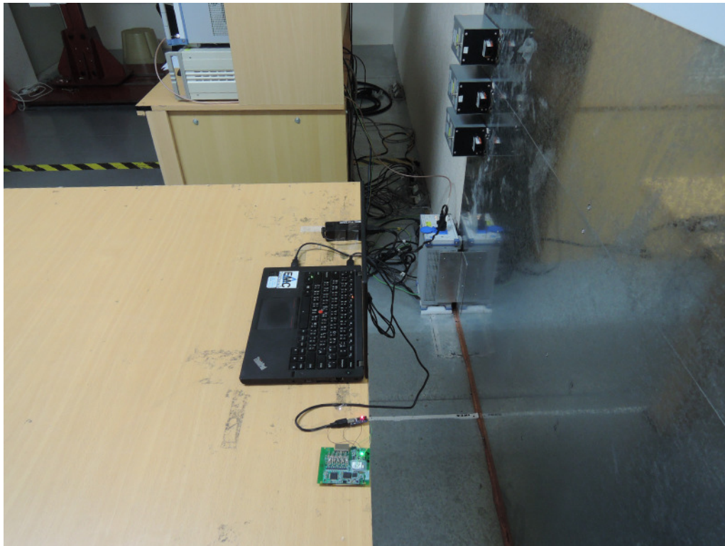
Photograph 6: Set-up for Mains Conducted testing (Back View)
