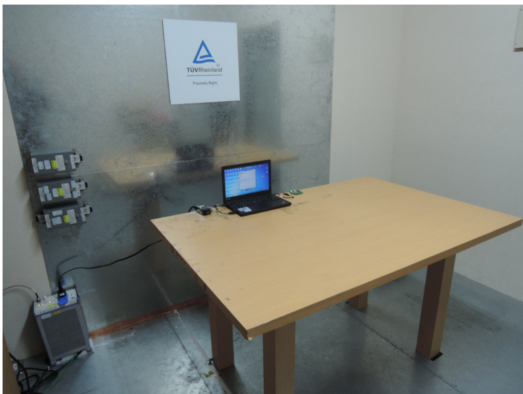
Photograph 7: Set-up for Mains Conducted testing (Front View)
