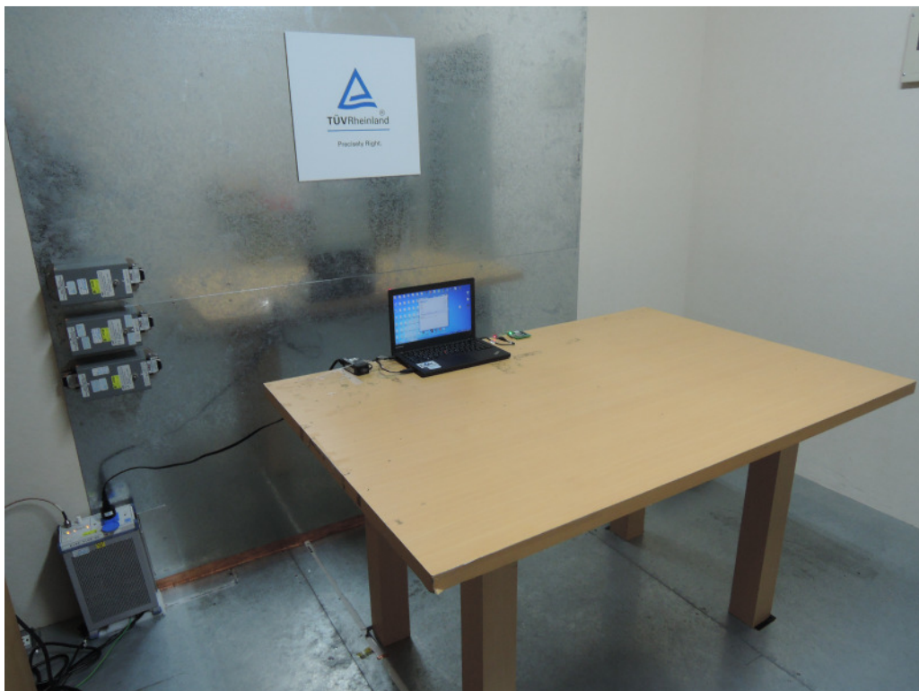
Photograph 7: Set-up for Mains Conducted testing (Front View)
