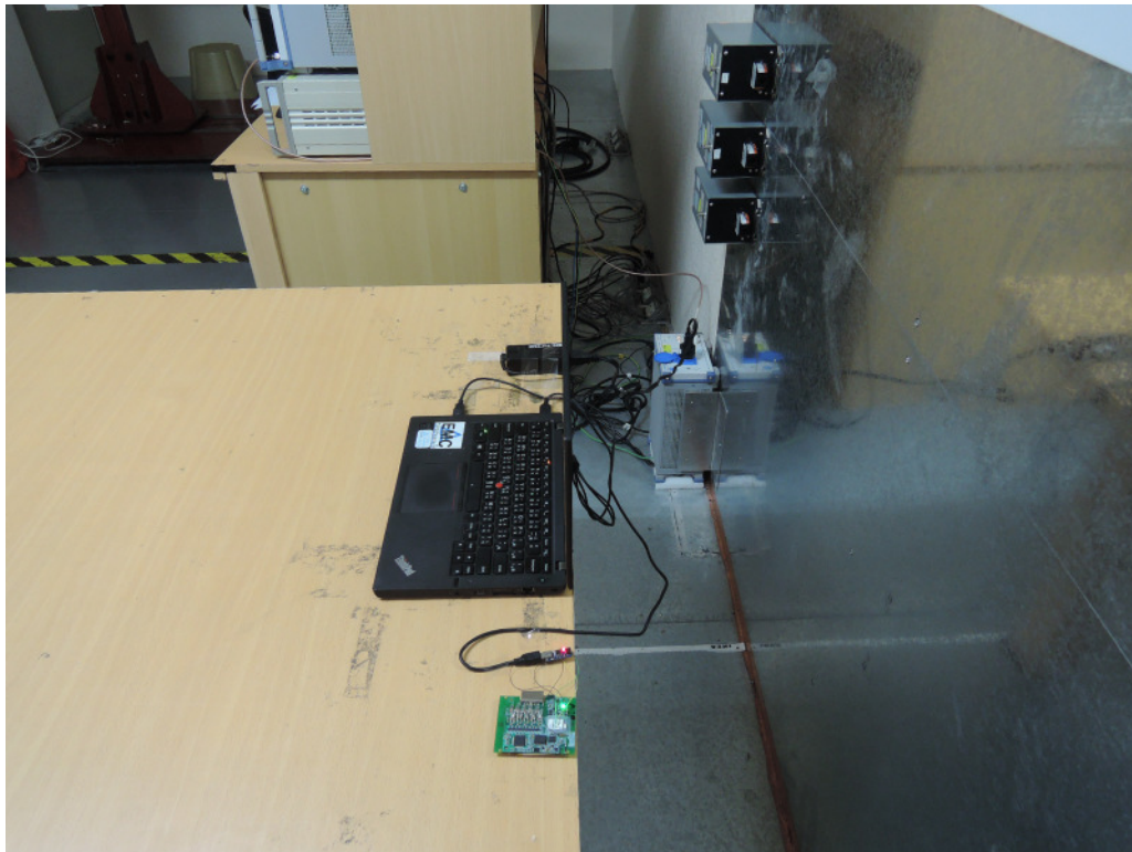
Photograph 6: Set-up for Mains Conducted testing (Back View)
