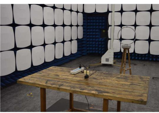
3. Radiated emission (9KHz-30MHz)
