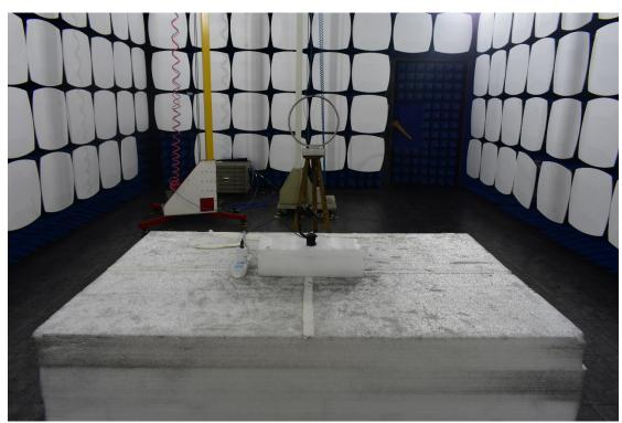
3. Radiated emission (9KHz-30MHz)
