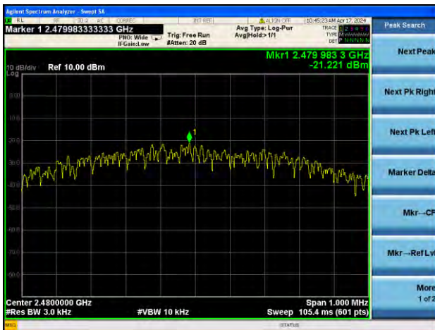
GFSK (BLE 1Mbps) HIGH CHANNEL
