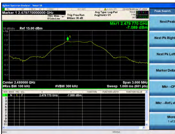
GFSK (BLE 1Mbps) HIGH CHANNEL, CARRIER LEVEL
