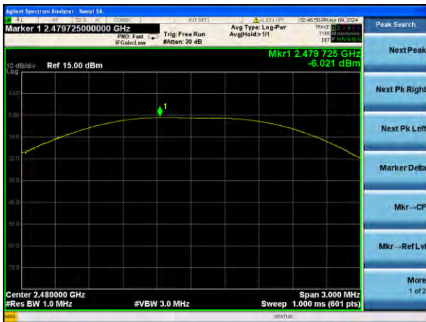
GFSK (BLE 1Mbps) HIGH CHANNEL
