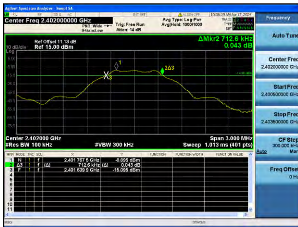
GFSK (BLE 1Mbps) LOW CHANNEL
