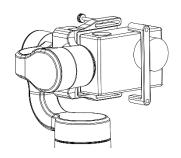
Put the tilt motor to the LEFT side, place GoPro 6/5 closely to the back clip as picture and tighten the knob to secure its position. Double tighten by 2 long screws against violent movement.
