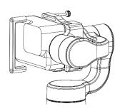
Put the tilt motor to the RIGHT side, place GoPro 6/5 closely to the back clip as picture and tighten the knob to secure its position. Double tighten by 2 long screws against violent movement.
