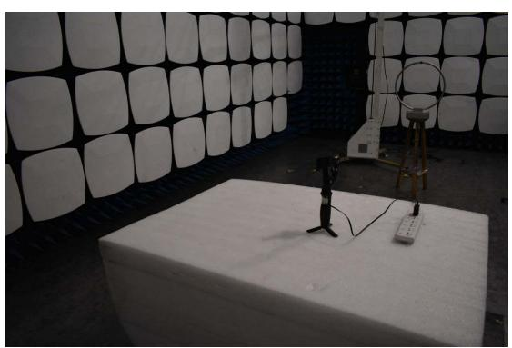
3. Radiated emission (9KHz-30MHz)
