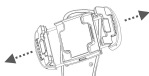
b. Pull the mobile phone clip to the max and make sure the charging port 2 and smartphone charging port are at the same side
