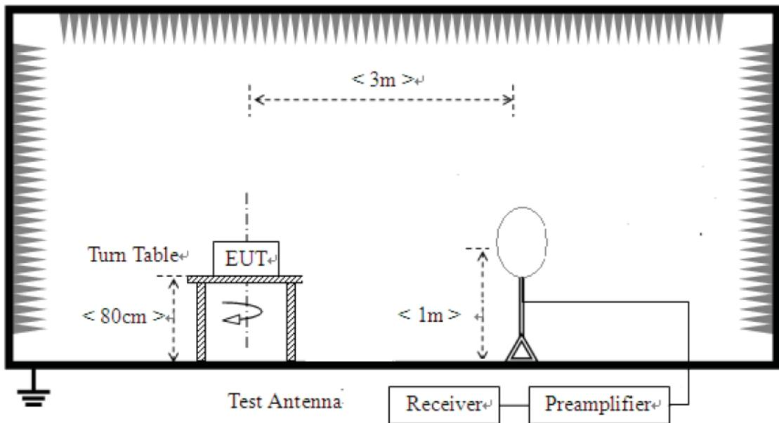
**Frequency measured at 30MHz to 1000MHz:**
