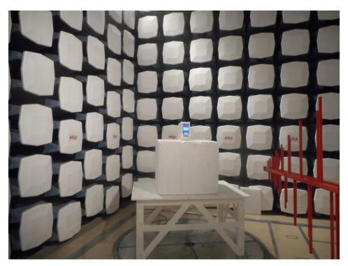
5.2 Radiated Emission below 1 GHz Rear View
