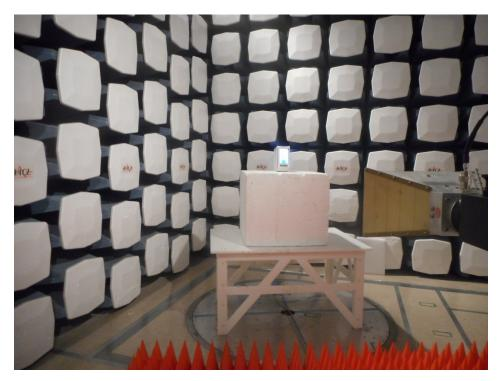
5.4 Radiated Emission above 1 GHz Rear View
