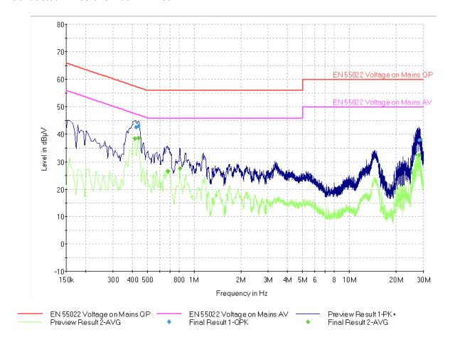
Note: Plots shown here represent the combined worse case emissions for power lines (phases and neutral line).
