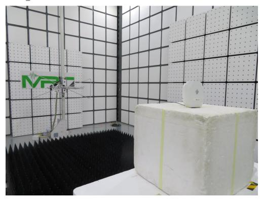
Description: Radiated Spurious Emissions Test Setup for above 1GHz\_OAW-AP1361D
