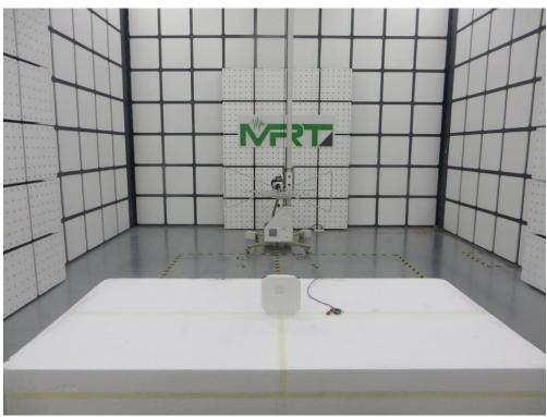
Description: Radiated Spurious Emission Test Setup for Below 1GHz
