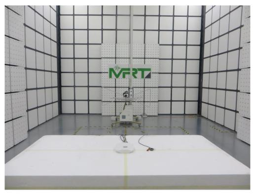
Description: Radiated Spurious Emission Test Setup for Above 1GHz Normal mode
