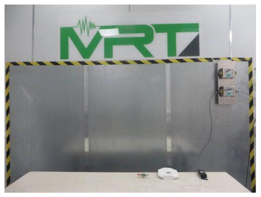
Test Mode 1 Description: Back View of Conducted Emission Test Setup for Power Port.
