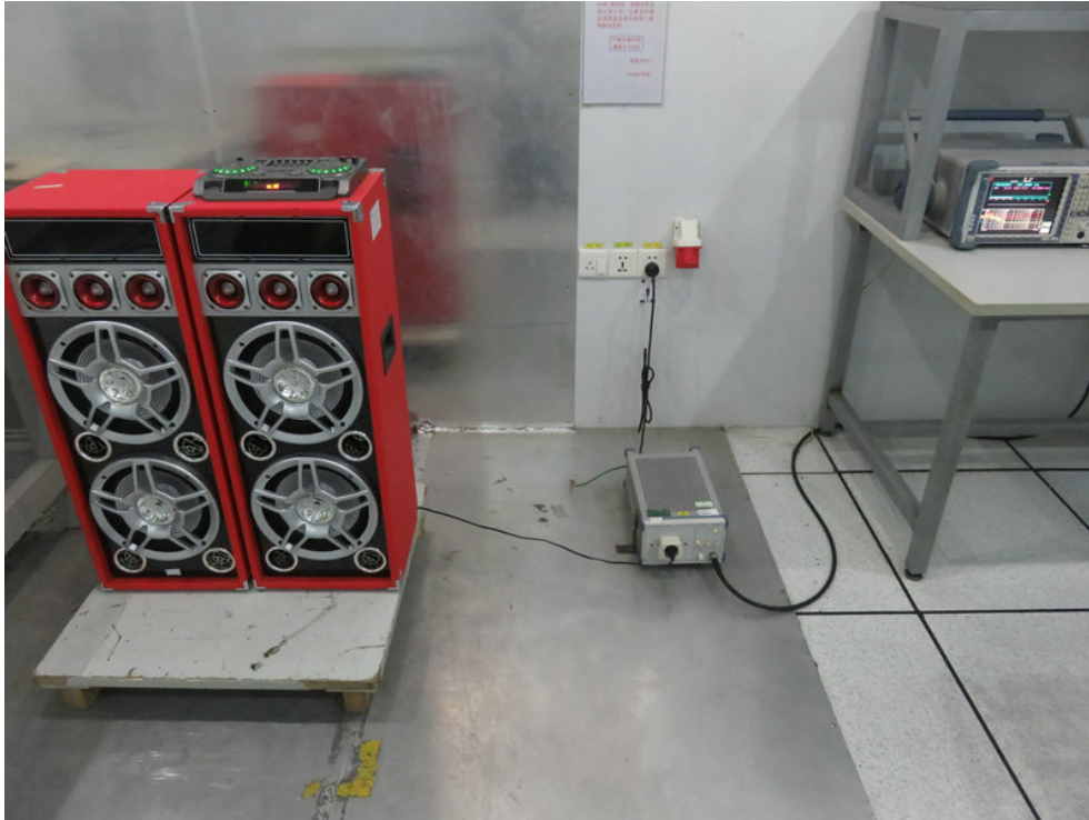
Photo of Conducted Emission Measurement
