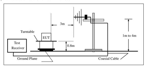
(c) For radiated emissions above 1000MHz
