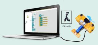
Camel F.1 uses USB cable to achieve program download or charge, when the robot is in charging, the LED on the USB side lights up red, when blue light up, it means that the charging is done. The charging voltage is 5V, and you can use the computer USB interface or other mobile charger to charge the robot.
