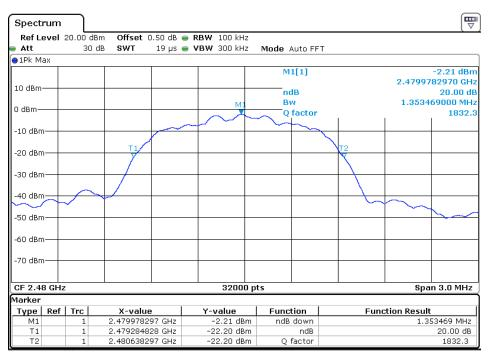
Modulation Standard: 8-DPSK Channel: 0
