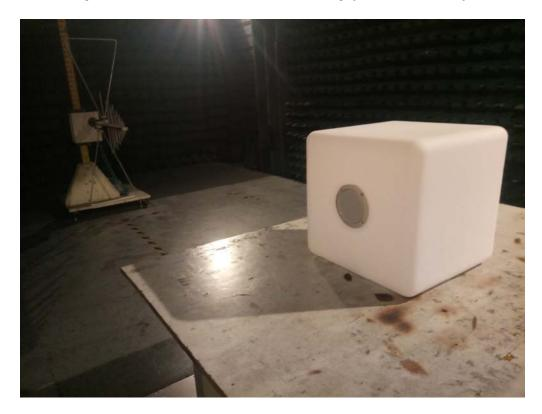
6.3 Radiated spurious emissions Test Setup(above 1GHz)
