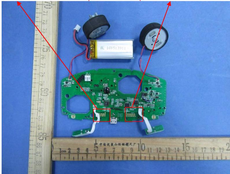
The Control software(AccessPort137.exe) can control antenna A/ B ,
