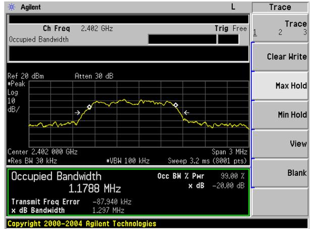
20dB Bandwidth plot on channel 39 (3Mbps)
