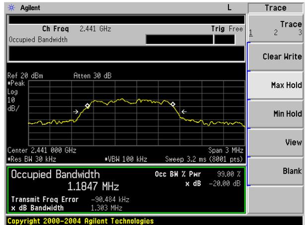
20dB Bandwidth plot on channel 78 (3Mbps)
