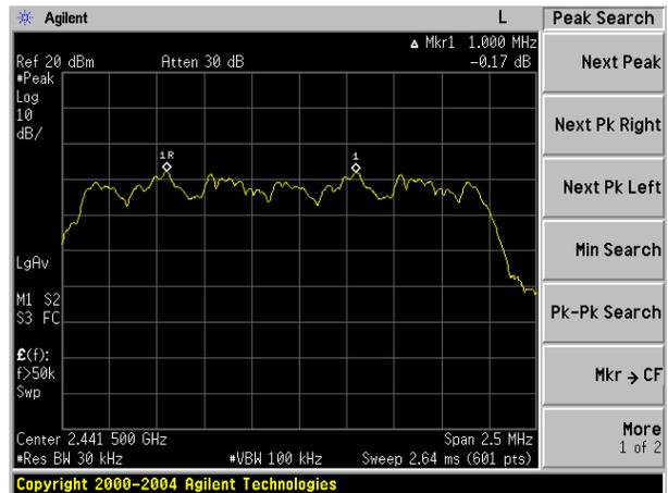
(3Mbps) Channel Separation plot on channel 77-78
