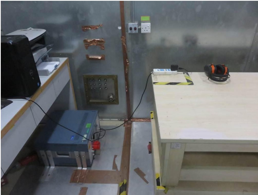
FCC RADIATED EMISSION TEST SETUP
