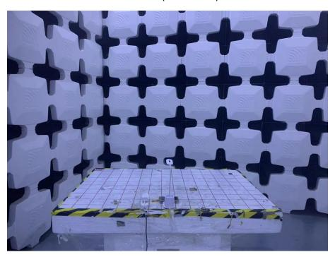
The EUT is placed at the center of turntable
