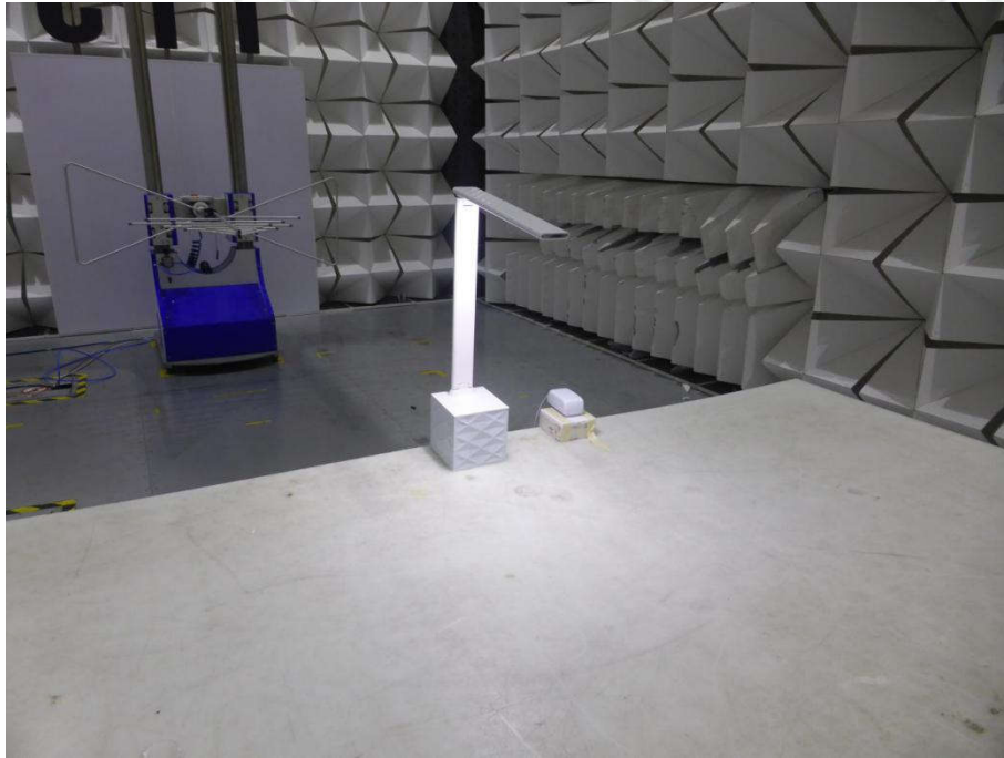
Radiated spurious emission Test Setup-1(Below 1GHz)
