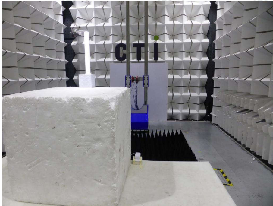
Radiated spurious emission Test Setup-2(Above 1GHz)
