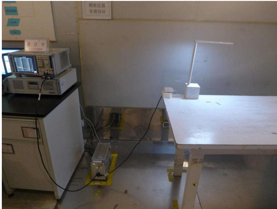
Conducted Emissions Test Setup
