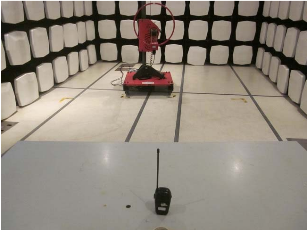
Measurement of Radiated Emission Test Set Up
