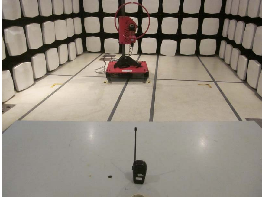
Measurement of Radiated Emission Test Set Up
