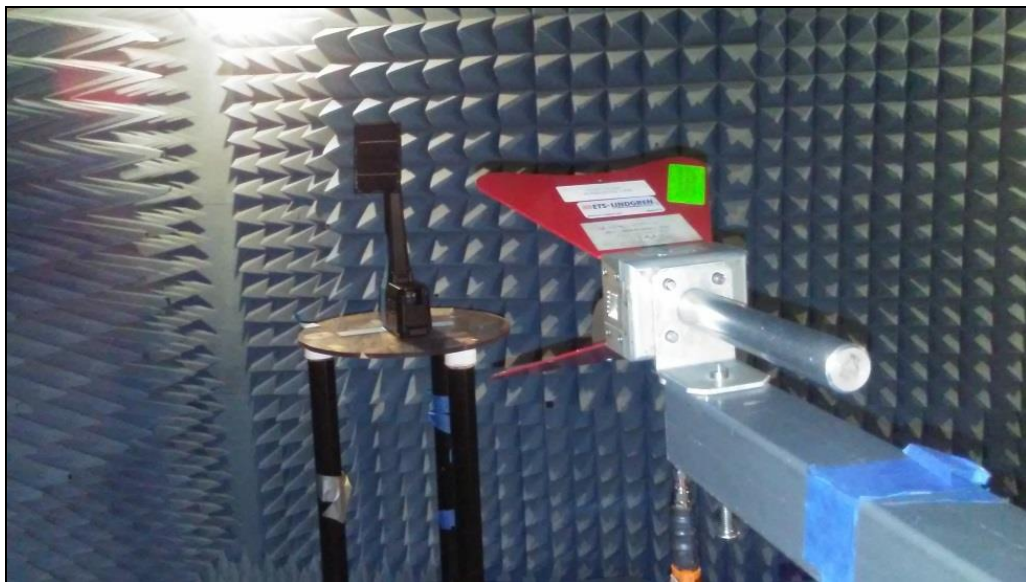
Photograph 2. Radiated Spurious Emissions, Test Setup, 1 GHz - 18 GHz
