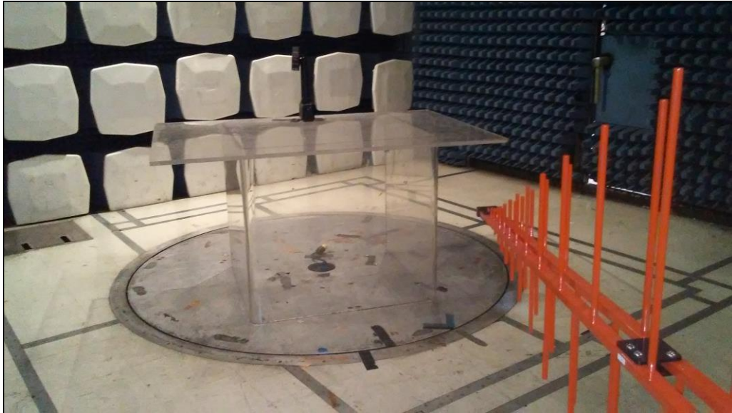
Photograph 1. Radiated Spurious Emissions, Test Setup, 30 MHz - 1 GHz
