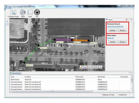
Figure 24: Screenshot showing a 'perimeter breach' alert and a 'node failure' alert
