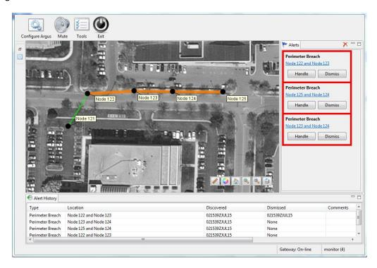
Figure 6: ARGUS GUARDIAN GUI in Active Mode. Alerts are shown in the right panel; Alert History is shown in the bottom panel, and current status is shown in the center Map View.
