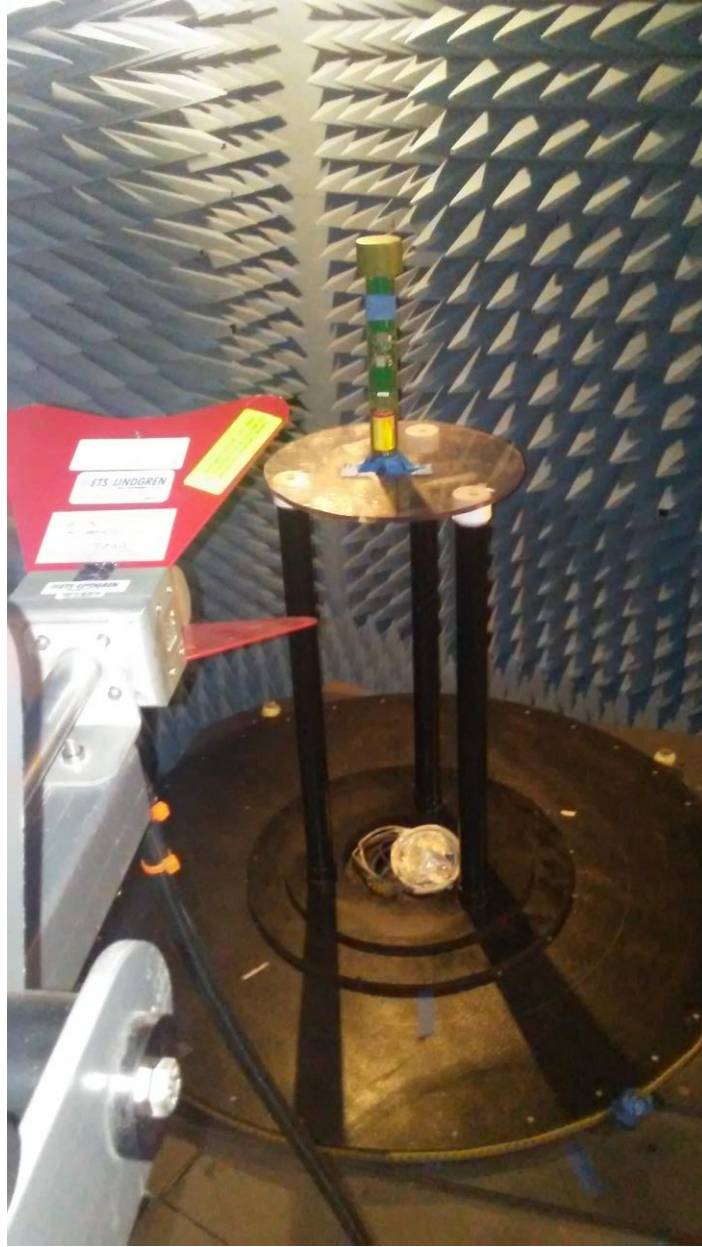
Photograph 2. Radiated Spurious Emissions, Above 1 GHz
