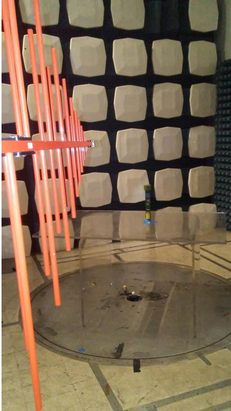
Photograph 1. Radiated Spurious Emissions, Below 1 GHz
