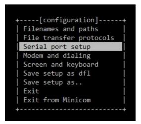
Go to Serial port setup and make sure the device is set according to the recognized USB device (in this case ttyUSB0). The rate is 115200 Bps and NO hardware flow control.
