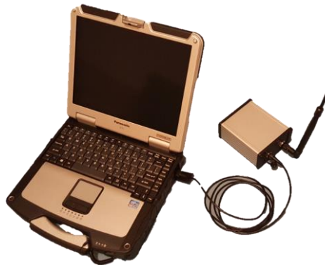
Figure 1: ARGUS Gateway connection to PC
