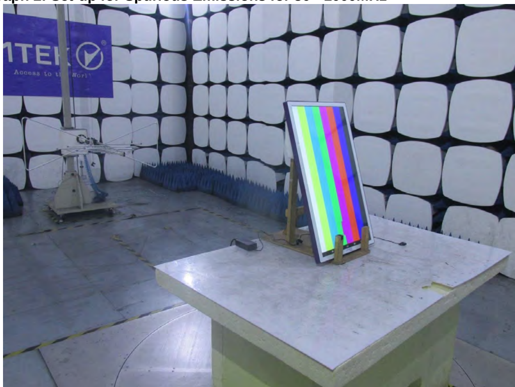
Photograph 2: Set-up for Spurious Emissions for 30 - 1000MHz
