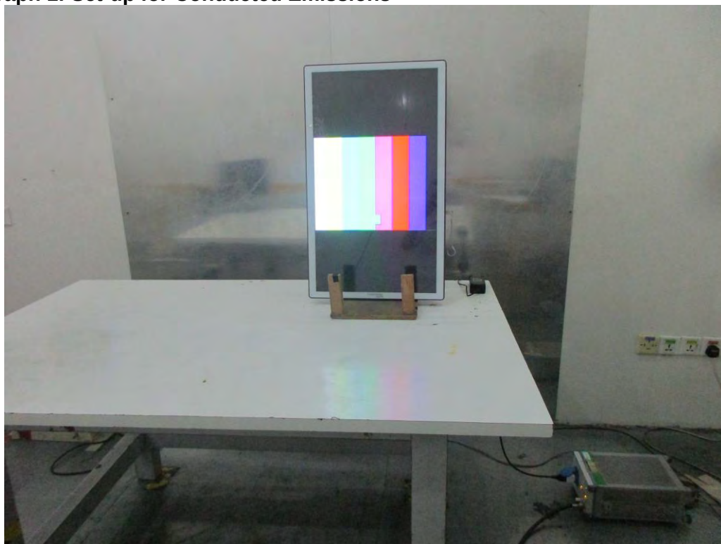
Photograph 2: Set-up for Spurious Emissions for 30 - 1000MHz
