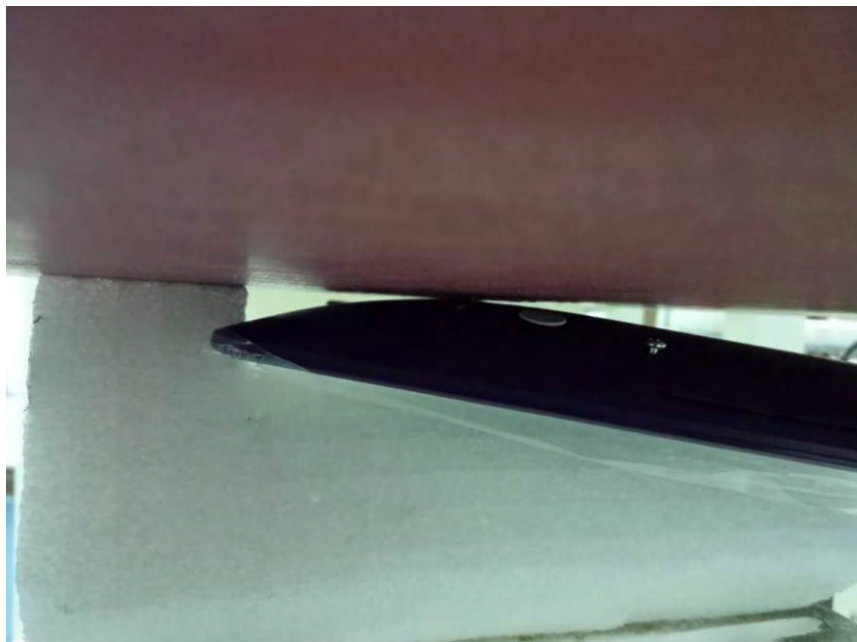
Photograph 4: Set-up for Back Face with antenna area contacted directly with Phatom
