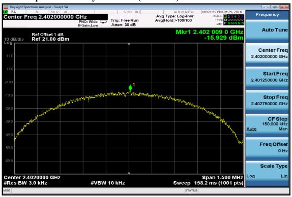
Power Spectral Density Test Plot (CH-Mid)
