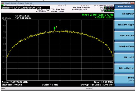
**Power Spectral Density Test Plot (CH-Mid)**
