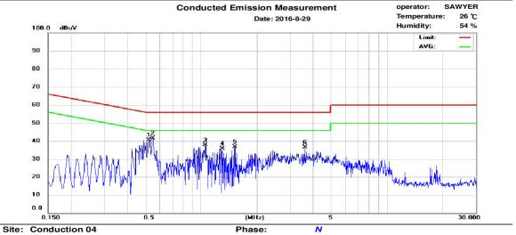
Limit: CISPR22 Class B Conduction(QP)
