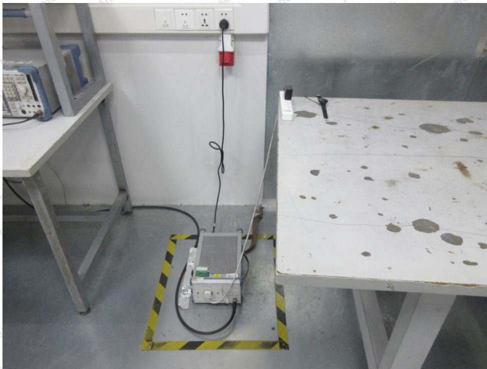
Photo of Power Line Conducted Emission Test
