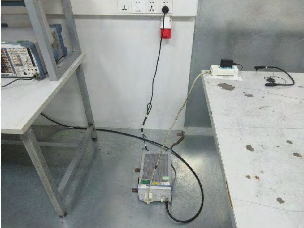
Photo of Conducted Emission Measurement
