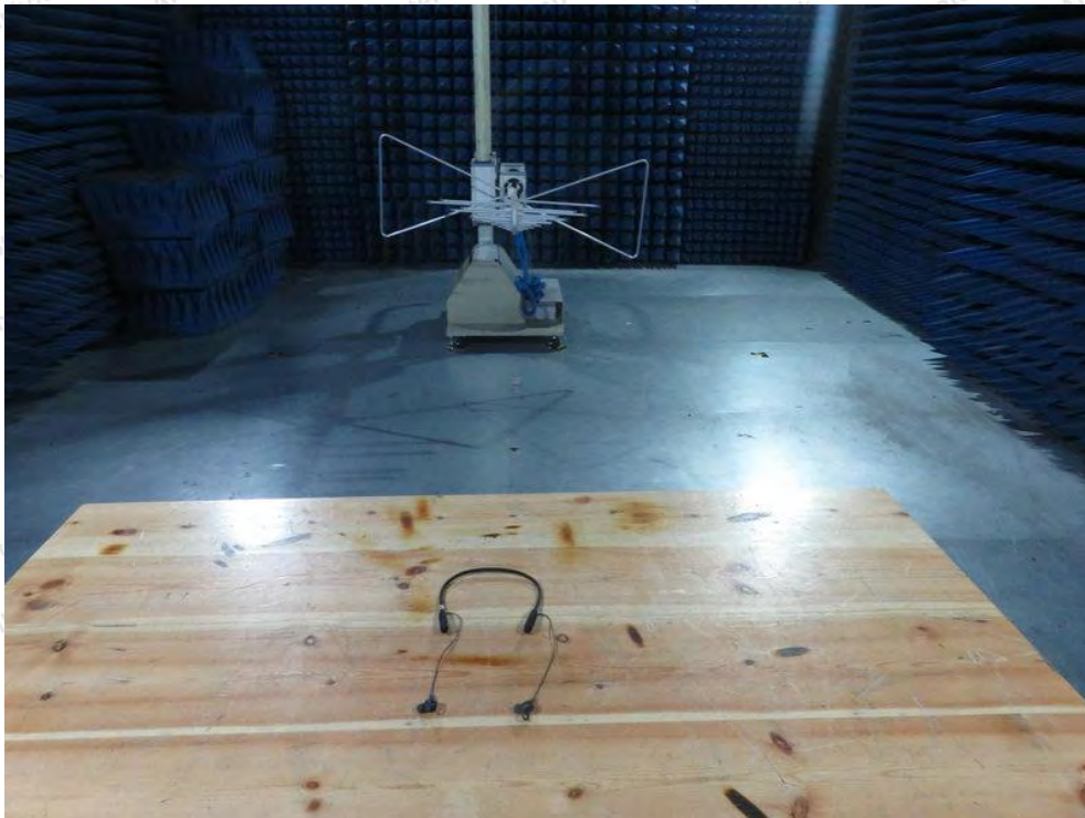
Photo of Radiation Emission Test
