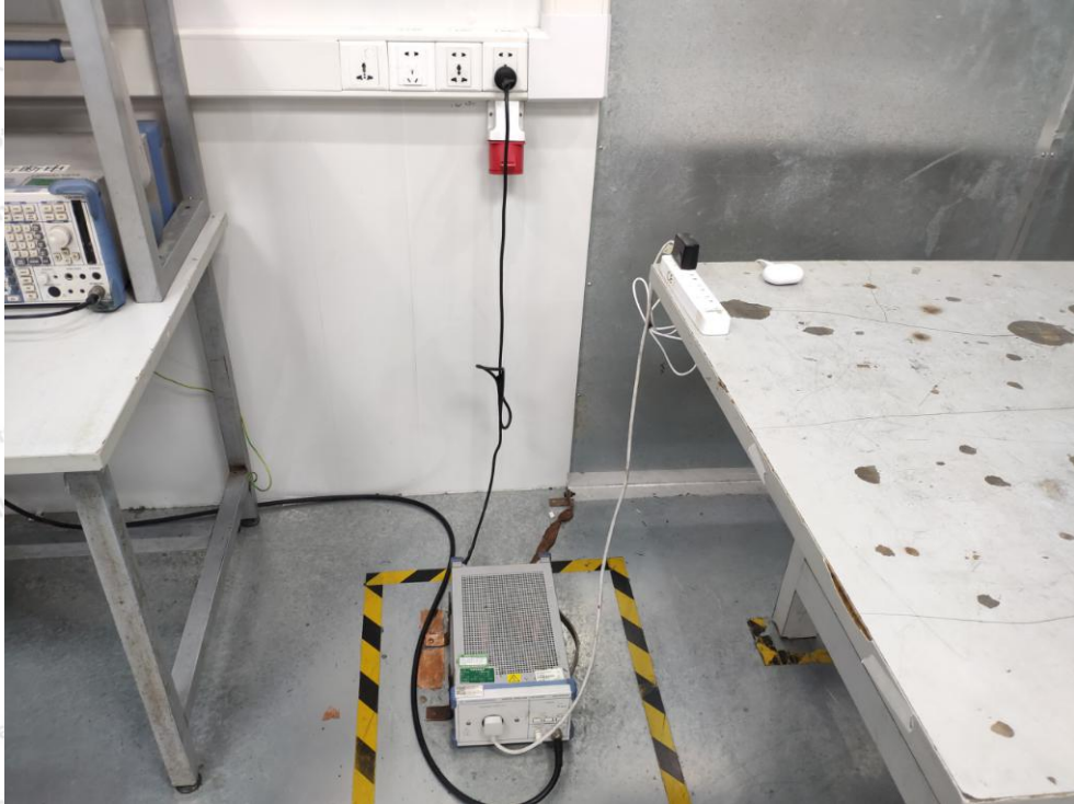
Photo of Conducted Emission Measurement
